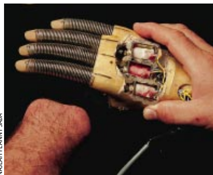
PROSTHETIC HAND allows flexing of single fingers when actuated by tendons or muscles.
